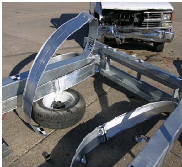
Figure 12. Damage from Medium-Speed Impact
