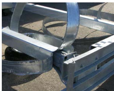
The mandrel cracks the energy absorbing tube at the corners and split it into four flat straps of metal.
