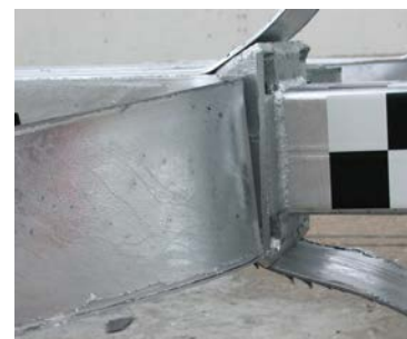
Close-up view of mandrel and energy absorbing tube.
